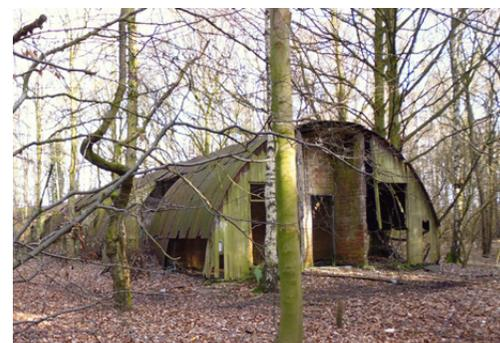
The Nissen Hut could be packed in a standard army truck and erected by six men in four hours. The world record for constructing one is 1 hour 27 minutes.
